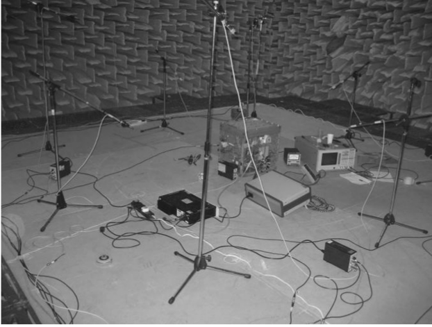
Fig. 3 Testing facility for the measurements of the sound radiation in the large anechoic chamber.
